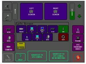
Figure 1. Complex AV Control System Interface
